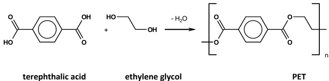
Figure 1: Structure and chemical equation of PET
